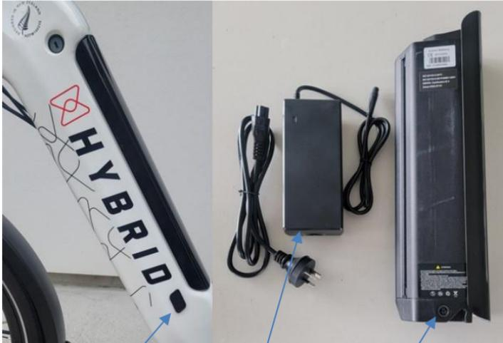
Charge point on frame    Charger    Charge point on battery
