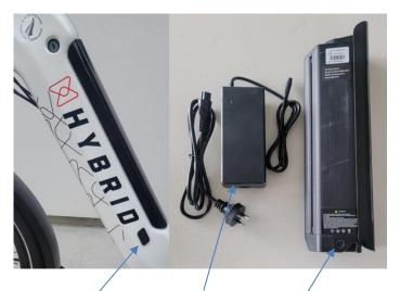
Charge point on frame Charger Charge point on battery
